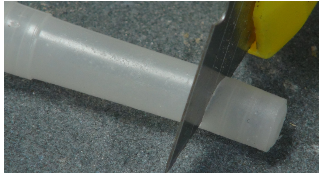
II. Cut half a centimetre of the lid.
