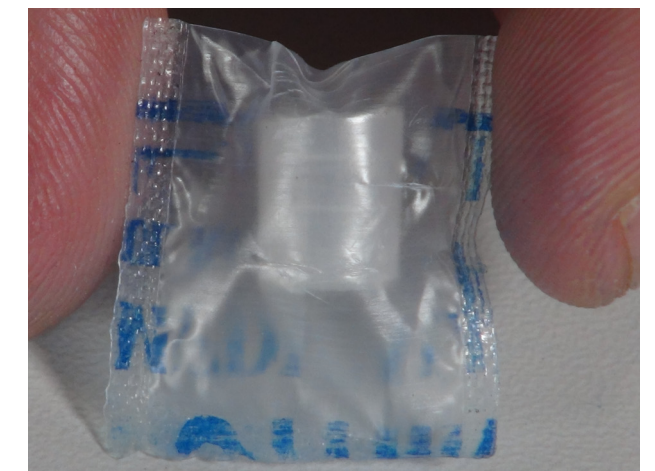
VI. Carefully place the acid-filled lid inside the bag. Do not pour the acid. Now seal the bag.
