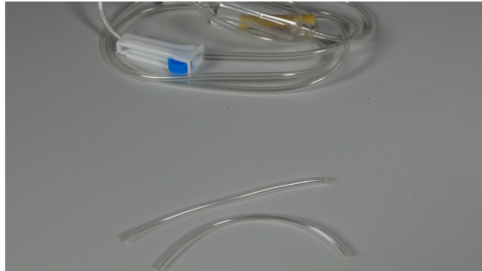
I. Take the pipe of a drip (medicinal drip). Cut it into two 10 cm pieces.
