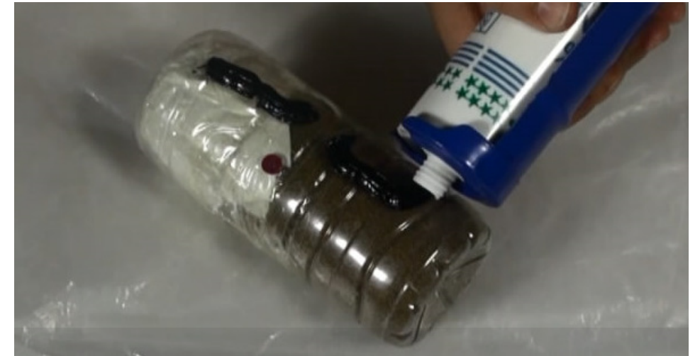
I. Apply a sufficient amount of silicone on the surface of the bottle.
