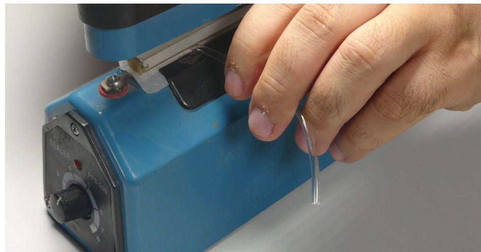
II. Take one 10cm pipe and seal one of the ends with a heat sealer.
