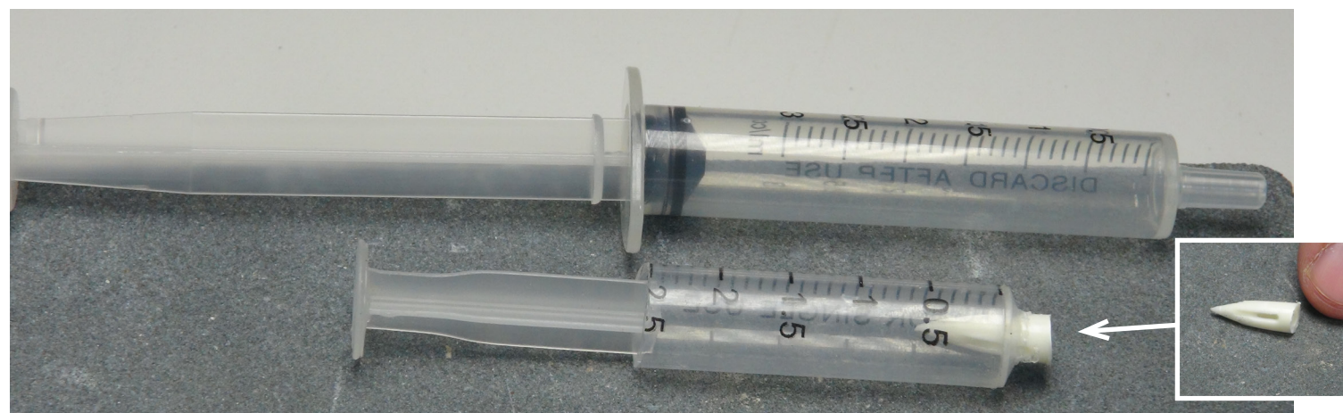
IX. Take a 3 ml syringe and cut it as illustrated above. Then make a hole in the bottom of the syringe and insert the plastic drip needle.
