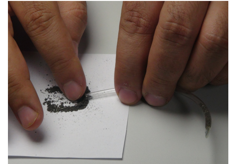
V. Fill the pipe with the mixture.
