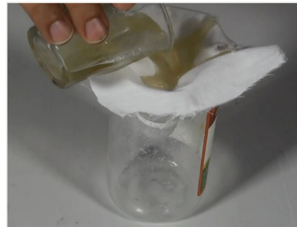
VI. Pour the mixture into the filter bottle. Dispose of the liquid.
