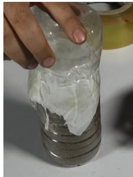
VI. Cut the base of another bottle and cover the first bottle.
