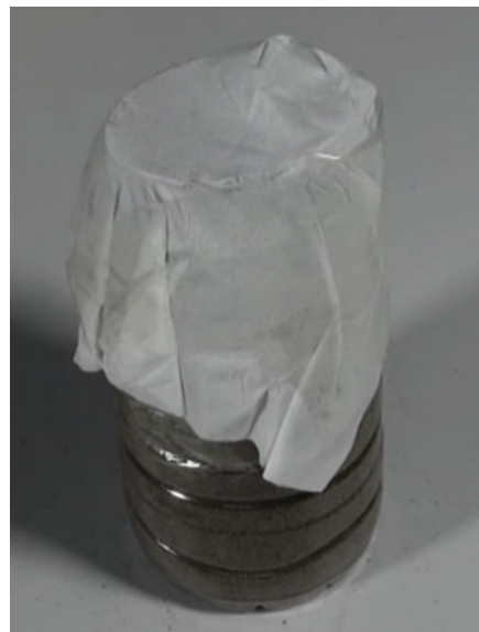
V. Place a tissue paper on the open side of the bottle, fasten it with a scotch tape.
